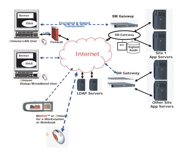
Using the **BioStik**™ with SecureMethods PKI solution; data is biometrically PKI secured and eliminates passwords by the user at the same time insuring identity.
